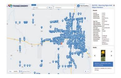
Results: The processed pavement evaluation and asset inventories are presented in the web-based Transconomy Viewer for dynamic visualization, and Geodatabase formats for flexible use by RCRPC.
