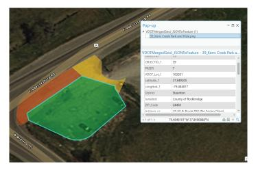
Transconomy successfully completed a comprehensive asset inventory and pavement condition survey of 127 P&R sites across Virginia. The project covered approximately 10.7 million square feet of pavement. The PASER analysis, encompassing asphalt, concrete, and gravel surfaces, provided critical condition data for near-term and future maintenance planning and prioritization. In addition to the PASER ratings, 26,000 parking spaces were inventoried, and the occupancy (parked cars) was noted.
